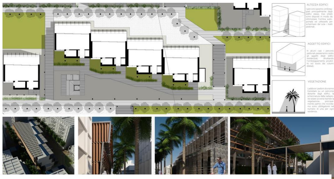
Fig. 6 - Project hypothesis of residential areas. The general plan and perspective views show the effect of the mutual sliding of the apartments to obtain sun protection and avoid introspection. This also allows, together with the vegetation, the shading of the pedestrian paths and common
