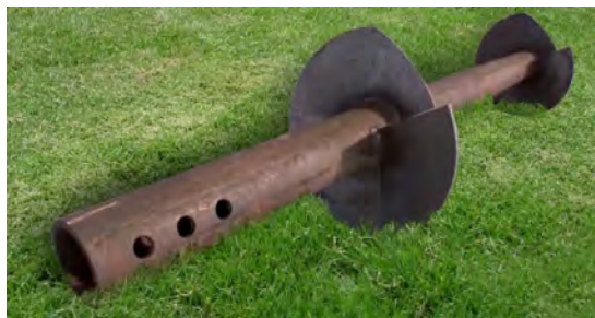
Fig. 15 - Upcycle House, Lendager Arkitekter - Nyborg, Denmark, 2013. Detail of foundation's pile
