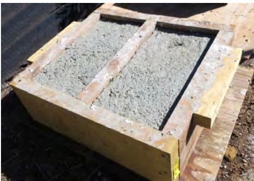
Fig. 6 - Bricks made of papercrete.
