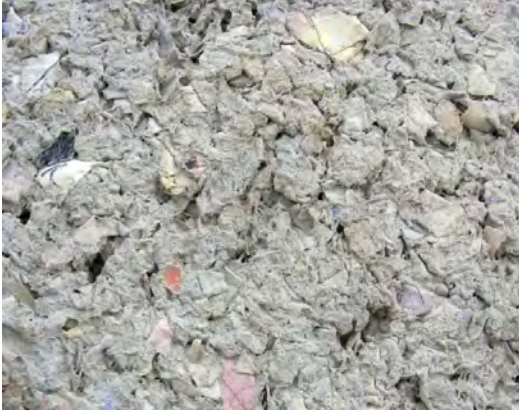
Fig. 5 - Papercrete, conglomerate made of paper, sand, concrete and water.
