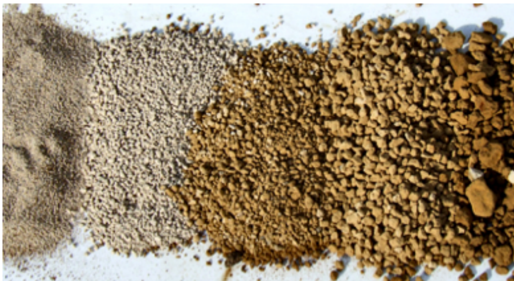
Fig. 2 - Different grain size of natural zeolites used in the RERARIA project (source: Ref. [14]).
