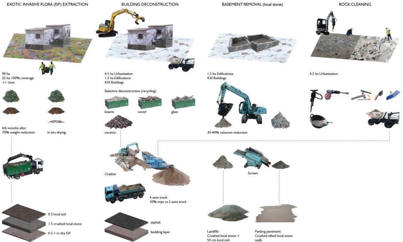
Fig. 6 - Tudela-Culip Restoration Project" (2010), Cadaqués, Girona, Spain. EMF Landscape Architecture: deconstruction and waste managements process. <a href="http://www.emf.cat">http://www.emf.cat.
