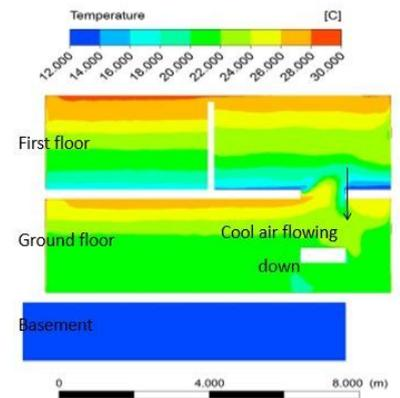
Fig. 5.b - A Top-down Cooling Design by CFD Simulation
