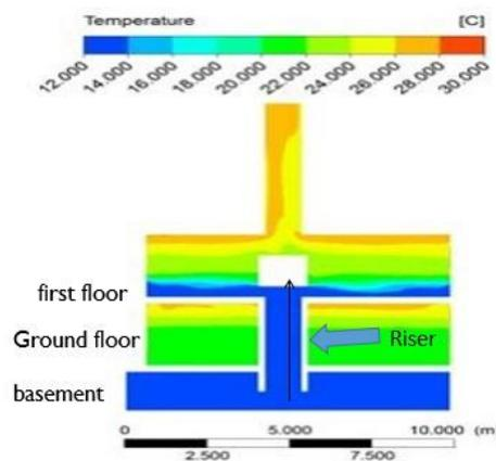
Fig. 5.a - A Top-down Cooling Design by CFD Simulation
