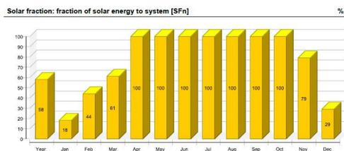
Fig. 9 - The Solar Thermal Energy to the System
