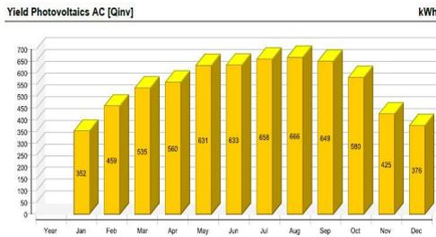
Fig. 7 - The System Photovoltaic Yield
