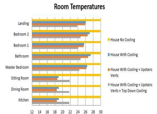
Fig. 6 - Room temperatures Results by CFD Simulation
