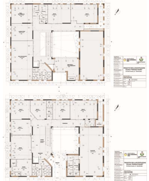
Fig. 6. Project of the new school "Romolo Murri" of Gualdo. Plan of the ground floor with the open space-cloister and a covered space-Agorà for socialization, 3 classrooms for primary school, a classroom for kindergarten school, a gym, a kitchen, a canteen, toilets, classrooms for middle schools, 2 laboratories, a multipurpose room, a teachers room, a library (source: L. Notarantonio 22/09/2017).
