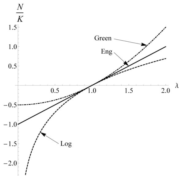
fig.03 - Graphs of three constitutive relationships, one linear (black solid line), the other two nonlinear (dashed line for the constitutive assumption with logarithmic strain, dotted-dashed line for that with finite Green's strain).
