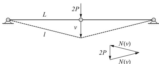
fig.01 - A two-bar mechanical system. The bars are assumed to be extensible.
