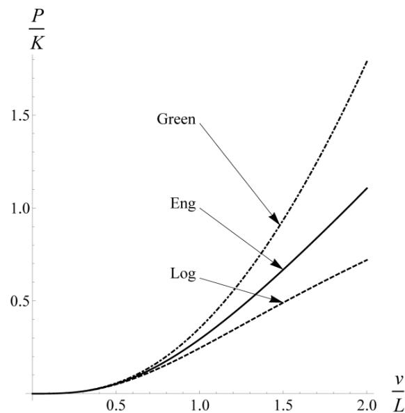
fig.04 - Nonlinear load-displacement curves: black solid line, dashed line and dotted-dashed line correspond to the engineering strain, logarithmic strain and finite Green's strain, respectively. Observe that also the curve corresponding to the linear strain is nonlinear, due to the geometrical nonlinearity of the problem under investigation.
