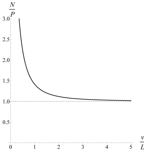
fig.02 - The variation of the dimensionless axial force as a function of the dimensionless displacement.
