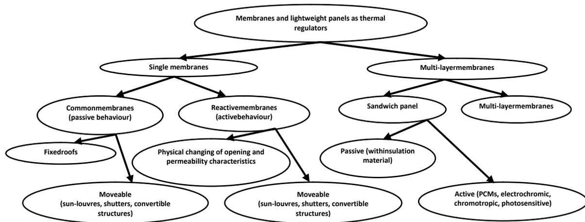
fig.01 - Classification of membranes and lightweight panels as thermal regulating elements [Mendonça, 1997]
