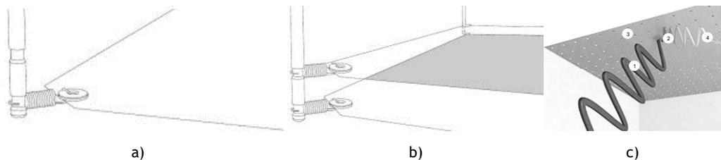
*fig.03 - Translucent and micro perforated membrane solution to improve the acoustic conditions of a compartment: (a) single membrane and (b) double membrane [Knippers et al., 2011]. (c) Scheme of reduction of the reverberation time of a perforated membrane: (1) Initial sound; (2) Transformation of sound into thermal energy; (3) Perforated membrane; (4) reduced sound [Barrisol, 2015]*
